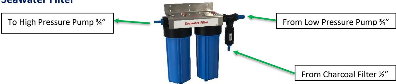
Mount the Seawater Filter near the Control Panel, leaving enough room below it to unscrew and remove the filter housing when cleaning. **Install new filters to each housing** as they are supplied empty. Water should flow through the 20 micron filter before the 5 micron filter (marked on blue ends). Install low pressure hoses as per diagram.
